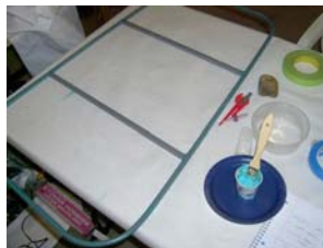
Figure 17-2 - Covering first panel, apply EkoBond to opposite side to be covered.
