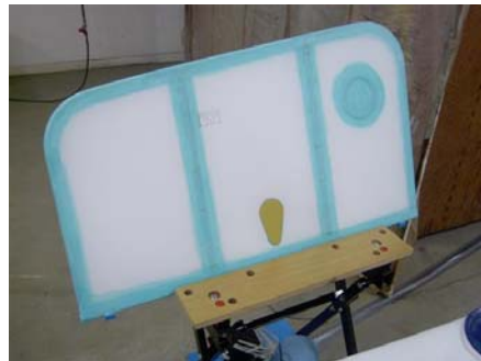
Figure 17-31 – Completed test surface ready for EkoFill.
