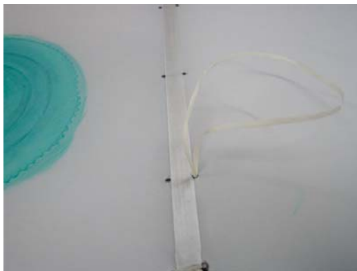
Figure 6-8 Forming loop for a modified seine knot.
