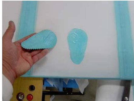
Figure 17-22 - Apply glue to fabric and patch.
