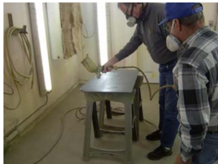
Figure 17-37 - Second spray coat of EkoFill.
