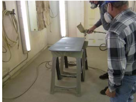
Figure 17-36 - First spray coat of EkoFill.
