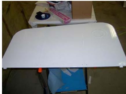
Figure 17-44 - Fourth coat with 2 nd cross coat completed.
