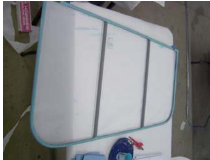
Figure 17-6 - Glue applied.
