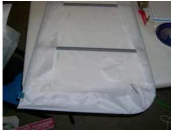
Figure 17-4 - First fabric panel in place and wrapped over frame.
