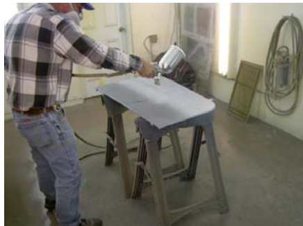
Figure 17-40 - First coat of 2 part topcoat (Insignia White).
