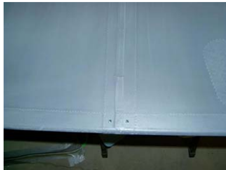
Figure 17-39 - Drain holes burned in with a soldering iron.
