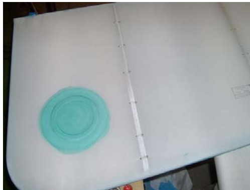
Figure 17-16 - Rib stitching complete.
