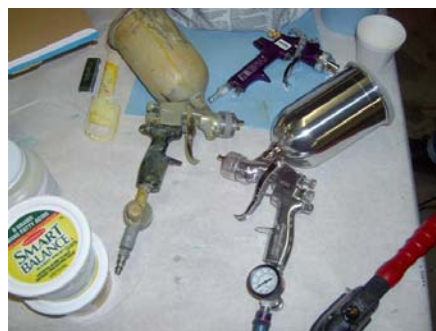
Figure 17-35 - DeVilbiss Finishline 3 spray gun with a 1.3mm tip.
