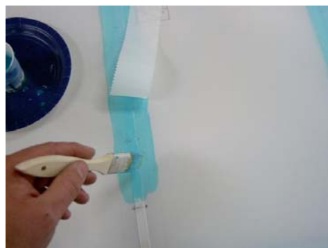
Figure 17-25 - Glue down tapes over rib stitch.
