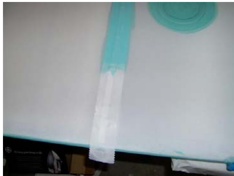
Figure 17-24 - Applying tapes over rib stitch.
