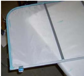
Figure 17-5 - First panel trimmed, applying EkoBond
