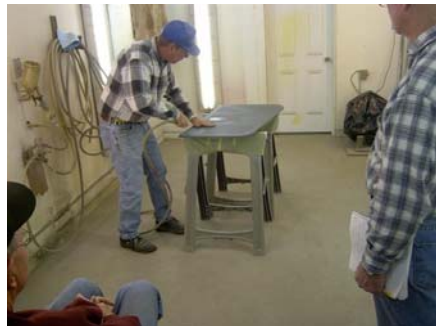
Figure 17-34 - Preparing surface by air blowing and wiping with a terry cloth.
