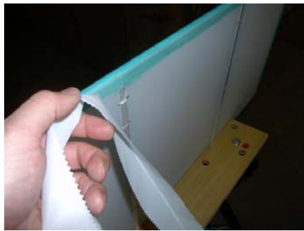
Figure 17-27 - Placing perimeter tapes on surface.
