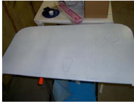
Figure 17-41 - First coat complete.
