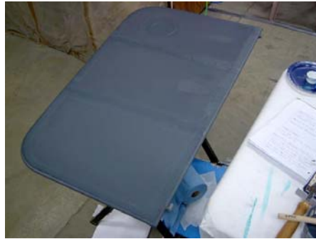
Figure 17-33 - Fabric surface after two brush coats of EkoFill and lightly sanded. Vacuum off or air-blow surface and wipe down with shop towel. See: Figure 17-34.
