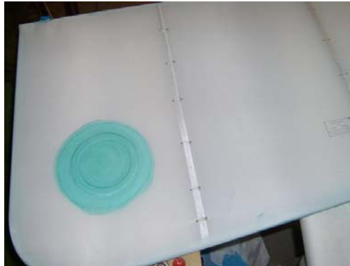
Figure 6-9 - Rib lacing complete.
