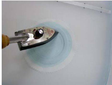
Figure 17-19 - Iron in the inspection ring patch.
