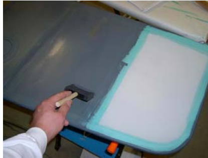
Figure 17-32 – Applying first brush coat of EkoFill Primer/UV Blocker/Filler.
