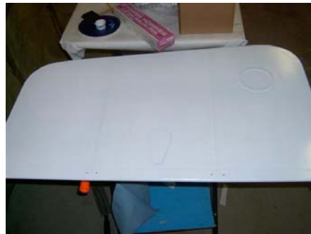
Figure 17-42 - Second coat with 1 cross coat completed.
