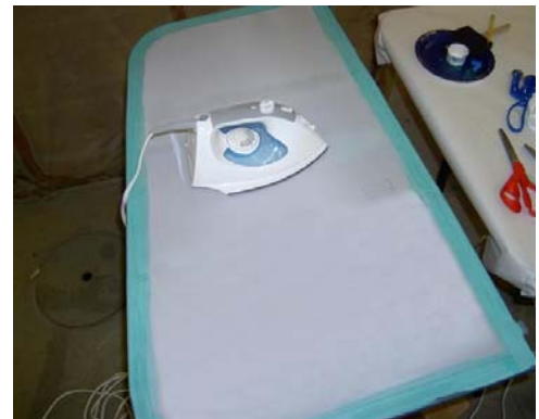
Figure 17-10 - Shrinking panel all the way to 350 ° F.
