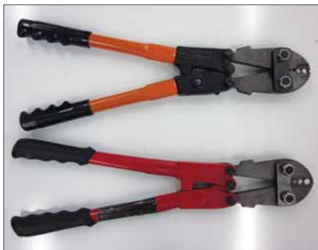
Fig. 15. A Nicopress 64-CGMP (top) and a $30 knockoff (bottom) may look the same, but the copy didn’t include a gauge and didn’t crimp to the correct dimension as delivered.
