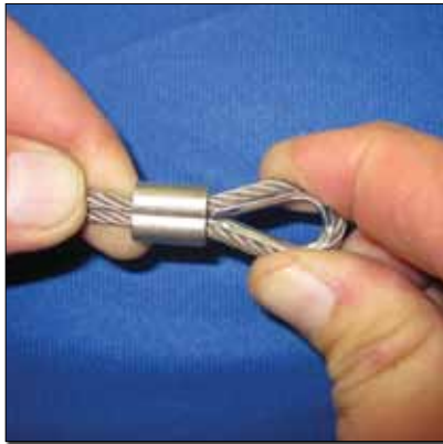
Fig. 8. Pull the cable tight around an AN100 thimble.
