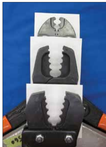
Fig. 17. Jaw openings of (from top) Nicopress CGMP, Continental/GBG S-2236H, and Locoloc 1-SC.
