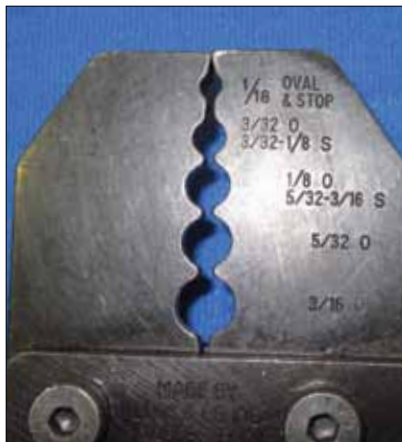
Fig. 13. Two of the grooves in the Locoloc 1-SC are marked with multiple fractional sizes. Note the “O” and “S,” which mean “oval sleeve” and “stop sleeve.”
