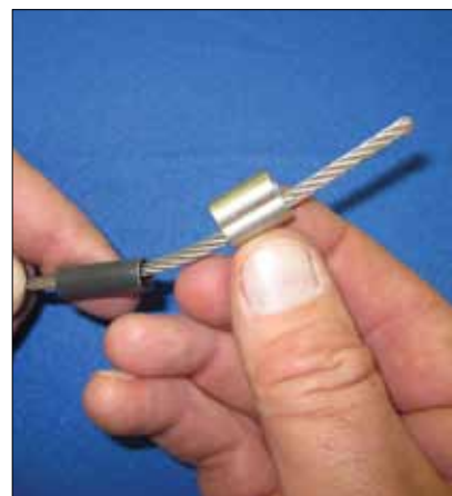
Fig. 6. Slip the cable through a short length of adhesive heat shrink, then the sleeve.
