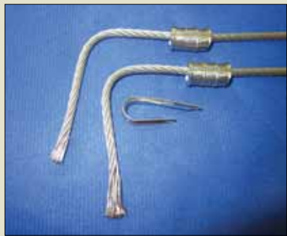
Fig. B. Under load, samples crimped larger than the gauge dimension often failed by pull-through, rather than cable failure.
