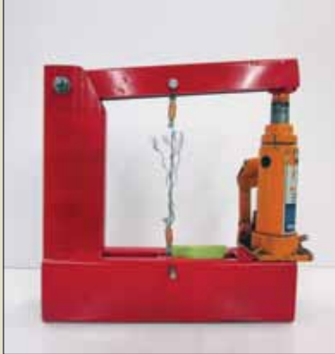
Fig. A. To examine performance at various crimp dimensions, multiple cable assemblies were crimped and pulled to destruction.
