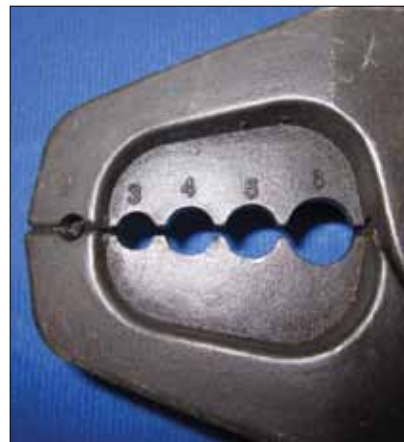
Fig. 14. For oval swage sleeves, the numbers on the Continental/GBG S-2236H jaws correspond to multiples of 1/32 inch. The same is not true for stop sleeves.
